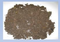
This waste has metallic contents that tend to be between 10 and 30%, mainly Cu, and in some cases Fe, corresponding the rest of the material to non-metallic fractions of low granulometry. Some particular filters are considered dangerous wastes due to their Pb content (> 0.3%); being difficult to treat, due to their fine granulometry and content of organic matter (20-30%) and inert (35%).
